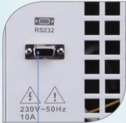
RS232 data interface for temperature monitoring (no software included)
