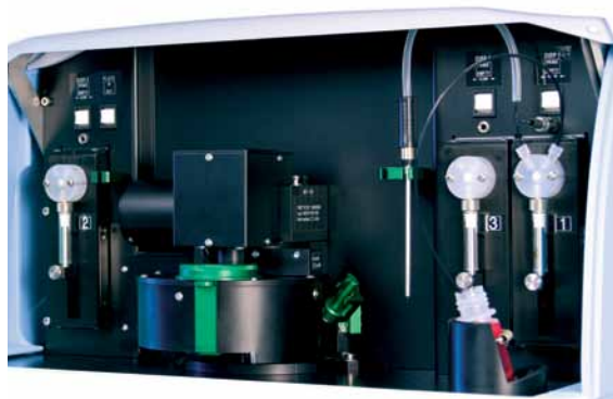
Onboard dispensers enable optimization of kinetic assays and facilitate assay development.
