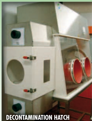
TRANSFER ISOLATOR CONNECTS ON ONE SIDE TO THE HOLDING ISOLATOR
