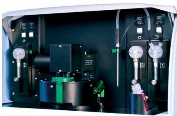
Onboard dispensers enable optimization of kinetic assays and facilitate assay development.
