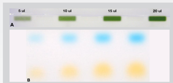
Figure 2. KapaTaq reactions with 1X Loading Dye Reaction Buffer A. Volumes above wells indicate the volume of the PCR reaction loaded on the gel.
