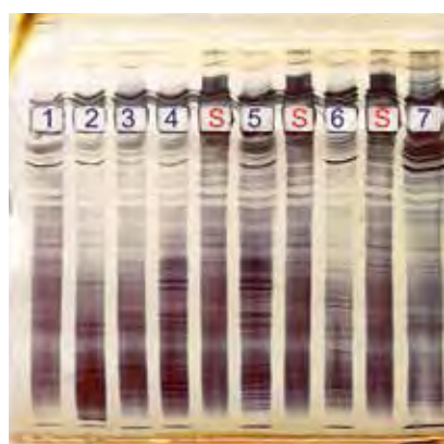
Serum/CSF analysis Comparison of CSF lanes (numbers) and serum lanes (S), separated on FocusGel 6-11, silver stained.
