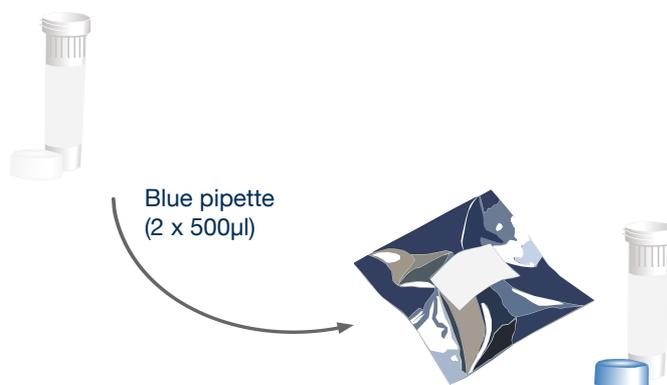
Use the blue pipette to transfer 1000µl (2 x 500µl) of water in to the Internal Extraction Control DNA tube. Cap and shake tube to mix.
