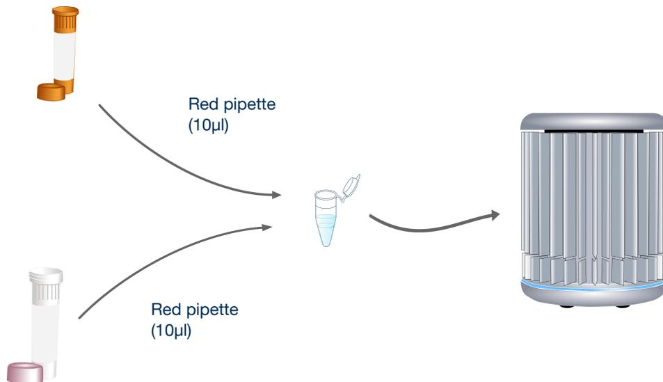
Take great care when setting up your positive control. The positive control template has the potential to give you a false positive signal in your other samples. Set positive controls up last after all other sample tubes are closed. Always change pipette tips between samples. You may even choose to set up positive controls in a separate room.
