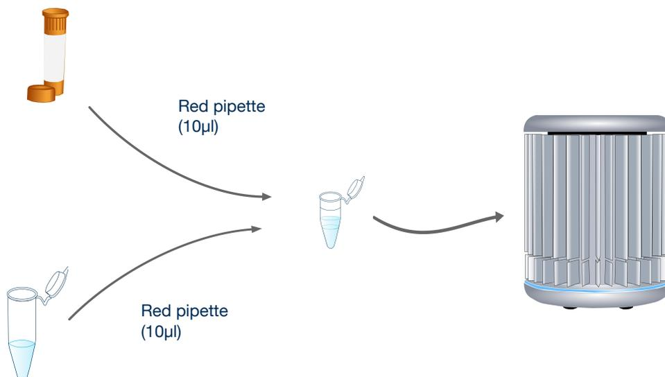
For each sample you wish to analyse, use the red pipette to combine 10µl of your Love Bird sexing reaction mix with 10µl of your DNA sample in the reaction tubes provided. Always change pipette tips between samples.
